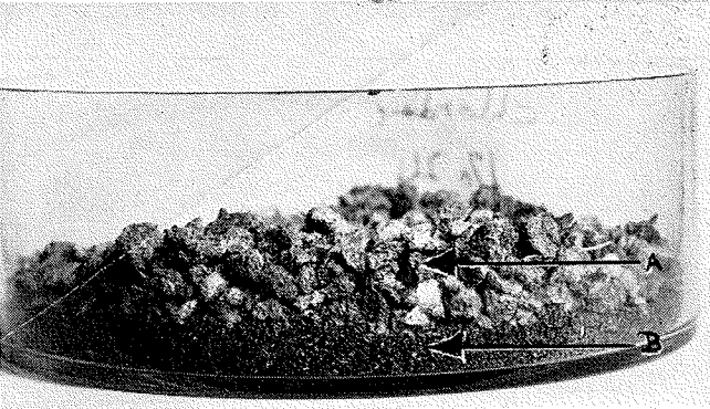
Figure 19. Type of large crystallization dish used in testing insecticides against arthropods under simulated natural conditions. Layer of dry chicken droppings (A) is always above layer of finely divided earth and feces (B), in which all stages of roaches and beetles are found.
