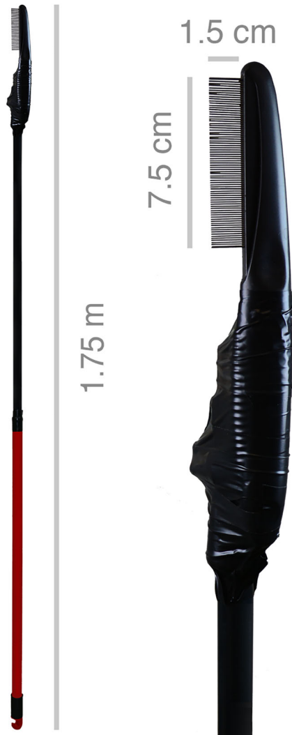
Fig. 1 “Telescopic lice comb apparatus”. Overview and close-up of the metal-toothed lice comb on the head of an aluminum telescopic rod fixed with Tesa® tape
