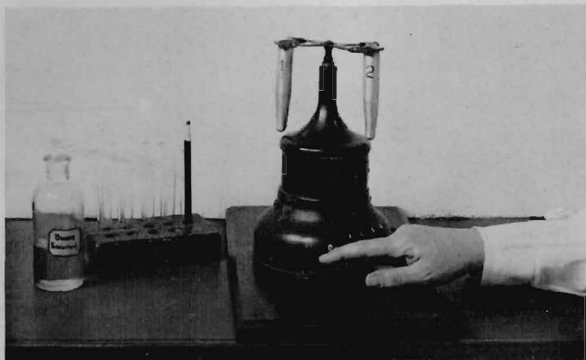
FIG. 9—Centrifuge the sample at approximately 1,500 revolutions for 3 minutes.
