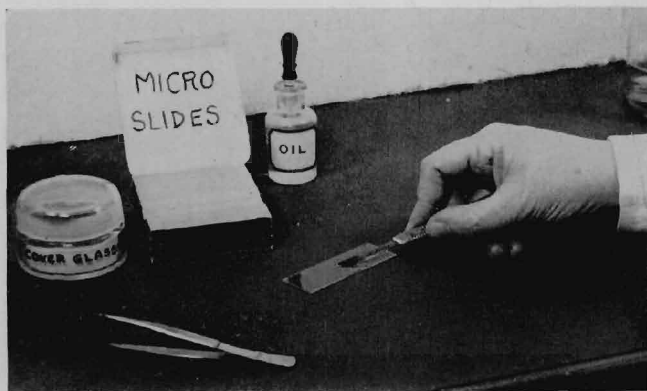
FIG. 197—Transferring the scraping from the scalpel blade to the drop of oil on the microslide.
