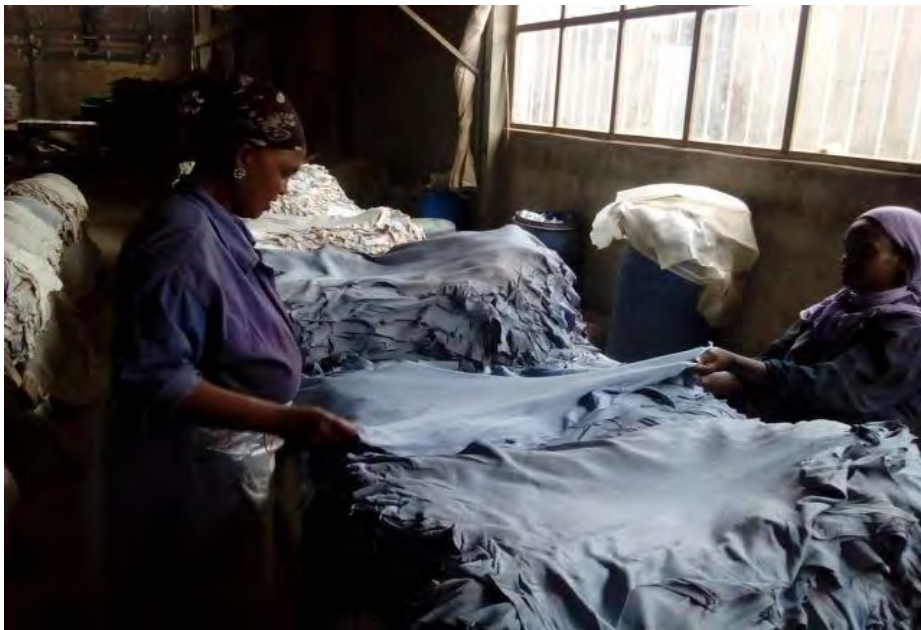
Figure 7: Observation of defects and grading wet blue goat skins in properly prepared and lighted point at Gelan tannery in Modjo
